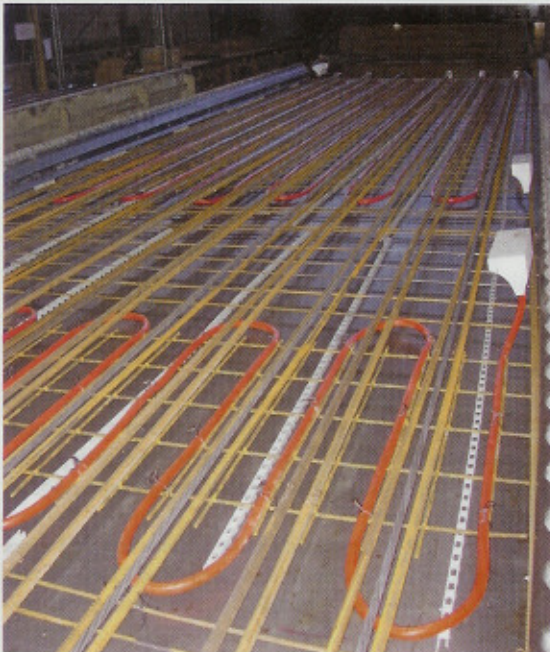
Fig. 2 A high-quality channel system is integrated inside the floor elements in the precast plant.
